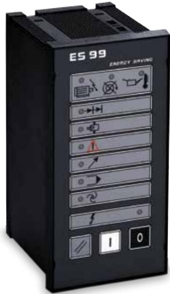
The ES99 offers you a straightforward control panel, providing a full set of warning messages to simplify your daily operations. Moreover, the ES99 software adjusts the load-no-load time to the actual consumption, preventing the electrical motor from running when it is not needed.
