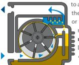
to a continuous film of oil. In this type of compressor no axial thrust is generated so the side surfaces of the rotor are not subject to wear and thus no rotating bearings or thrust bearings are needed. The vanes, too, because of the special way they are
