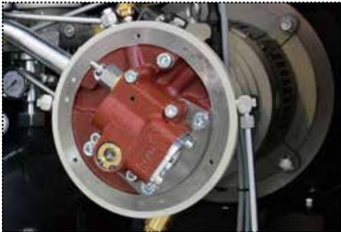
When there is no air demand for short periods of time, the on/off load valve allows the compressor to **significantly reduce its internal pressure thereby reducing energy consumption to a minimum**, without having to stop the compressor. The number of stops and subsequent starts is therefore reduced, which **helps increase the life span of the compressor and its electric motor**.
