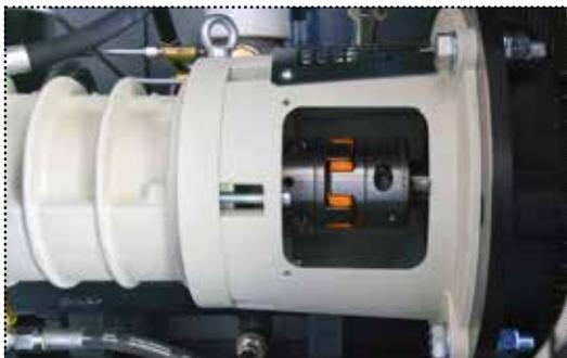
BLADE 8-12 i has been designed in a way that makes it possible **to replace the elastic element** without having to dismantle the rotor-stator unit.
