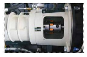
BLADE 8-12 has been designed in a way that makes it possible **to replace the elastic element** without having to dismantle the rotor-stator unit.
