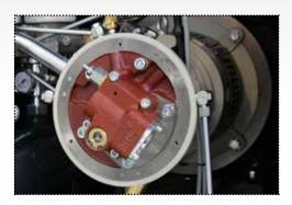
When there is no air demand for short periods of time, the on/off load valve allows the compressor to **significantly reduce its internal pressure thereby reducing energy consumption to a minimum**, without having to stop the compressor. The number of stops and subsequent starts is therefore reduced, which **helps increase the life span of the compressor and its electric motor**.
